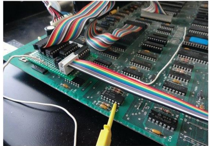
FIGURE 8. Final P2P board mounted on video connector, ribbon cable to latch (top), white wire to remap RAM, and yellow clip to border blank signal.
